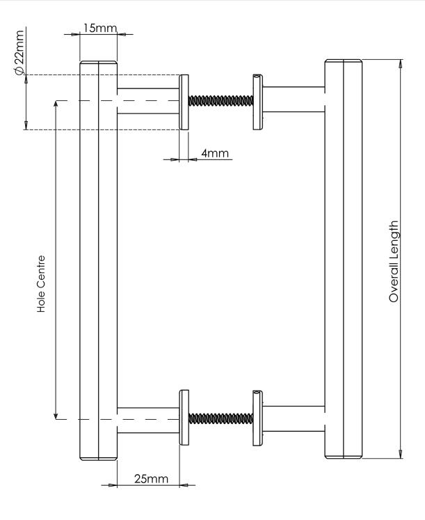
**NOTE:** All dimensions are in MM. Protective lacquer applied to prevent oxidisation and corrosion. Suitable for all appliance doors.
